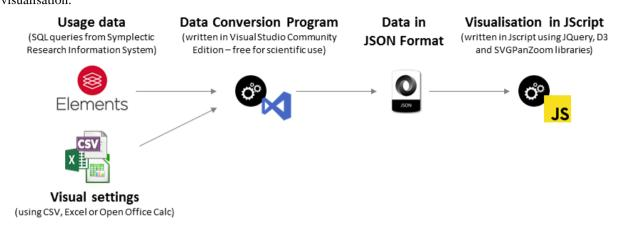
Fig. 1: Framework for data loading and staging
