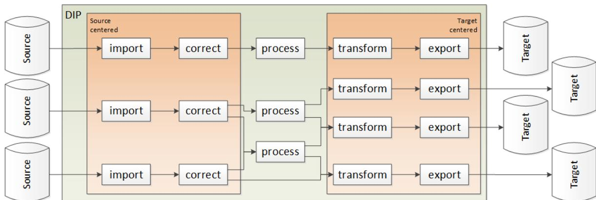
Fig 1: Data Flow Architecture.
